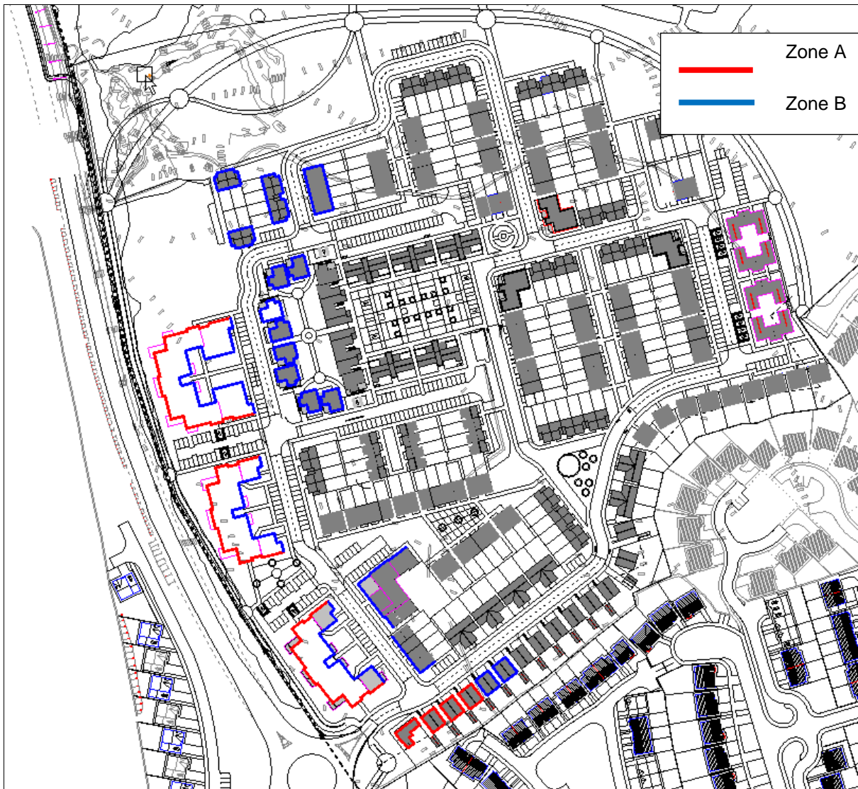
Figure 9.12 Façade zoning for noise mitigation measures
